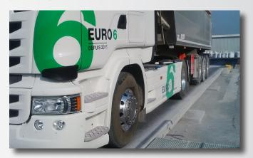
As it is modular the ROC weighbridge can perfectly be adapted to meet your needs. Sizes range from 4m to 24m in length with a standard deck width of 3m. Other sizes are available on request. As it is composed of between one and four precast concrete decks ROC offers a uniquely strong yet portable weighbridge.
